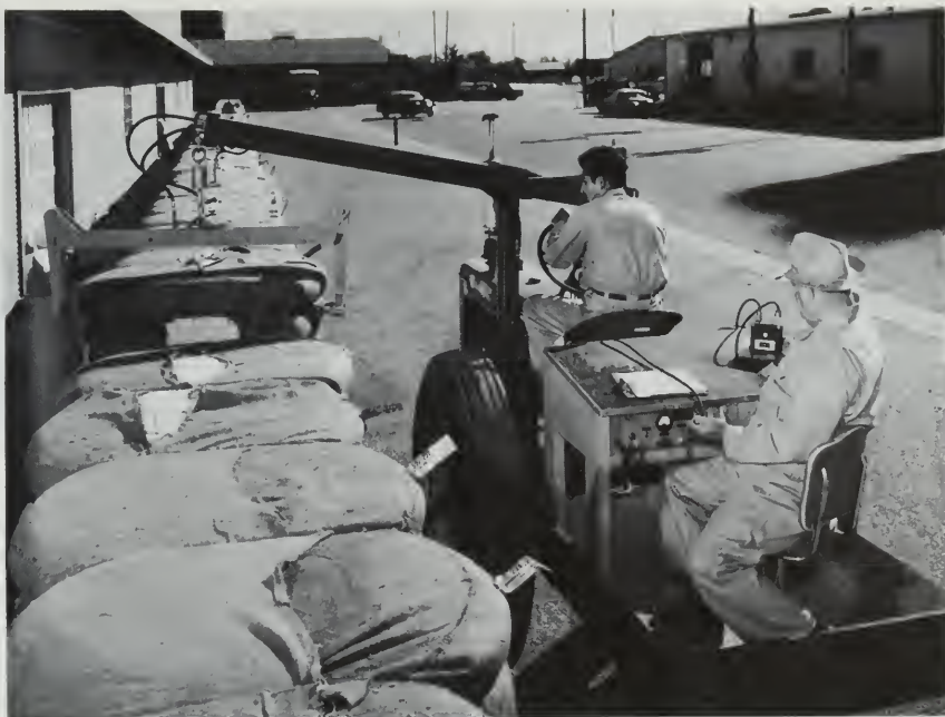
An electronic scale for weighing cotton does the work once done by 14 to 20 men.
